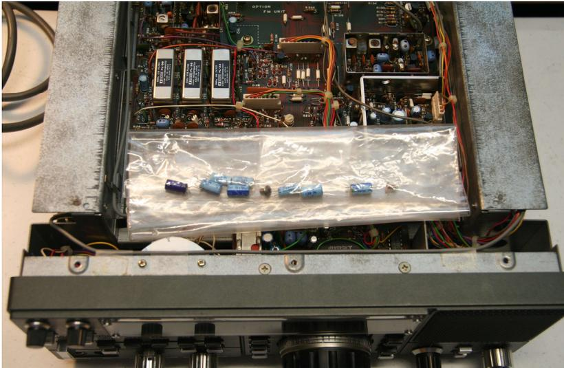
With covers removed, I take a quick look for burnt components, missing parts, disconnected leads, bulging electrolytic capacitors etc. Finding none, I suspect there is a glimmer of hope this Receiver is repairable. I also note this Receiver has an optional InRad SSB XTAL filter in 455 KHz IF section!
