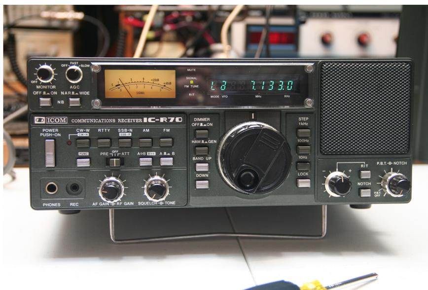
Checking all of the modes and functions, I notice a significant pitch change when shifting from LSB to USB so there are likely more alignment issues, possibly with the BFO or the pass band tuning circuits, which need to be dealt with. I'll get to those when I have another day with no other pressing projects.
